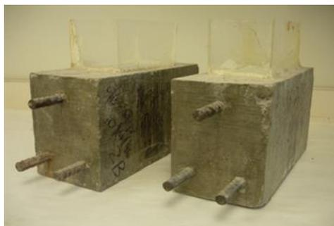
Figure 6. Example of ASTM G109 Test Blocks
