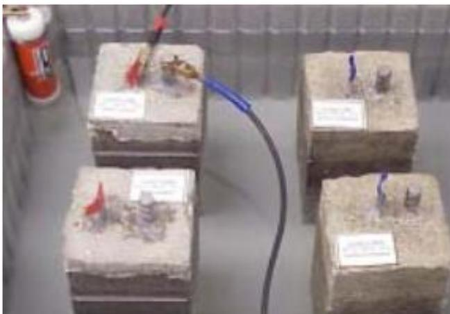
**Figure 16. Modified ASTM G109 Test Set-up (continuous submersion)**
