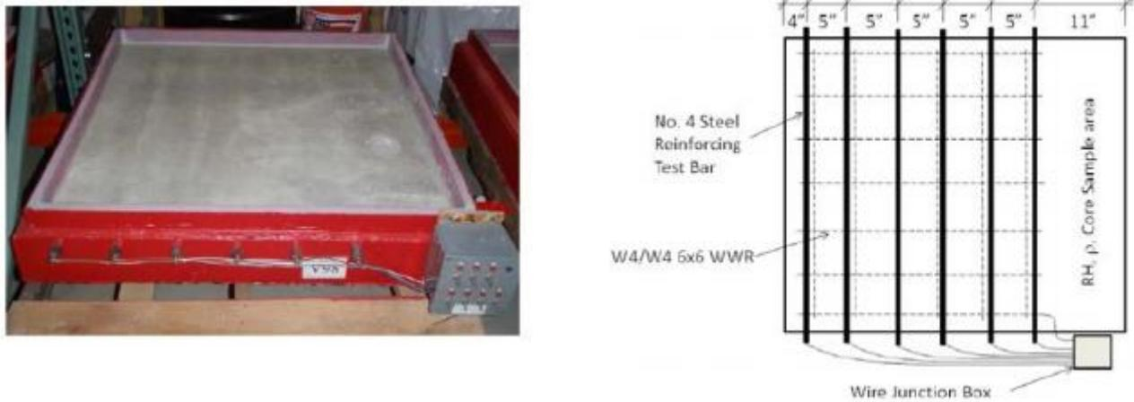
**Figure 10. Photo and Bar Layout Diagram of M-82 Test blocks**
