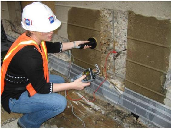
**Figure 22. GalvaPulse Readings Prior to Repair**
