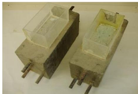
Figure 7. Example of ASTM G109 Test Blocks
