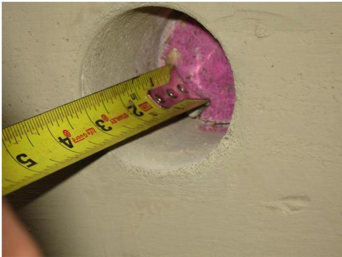
**Figure 18. Carbonation Testing on Lightwell Wall**
